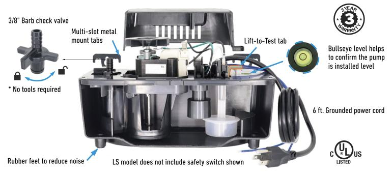
New design offers a longer 3 year warranty life and reduced noise level. Includes lid mounted bullseye level for easy installation. Rated for condensate water up to 150° F. Automatic start/stop operation with thermally protected motor. More water pumped out per cycle means the pump runs less and lasts longer. Larger 2.5 quart tank capacity.
